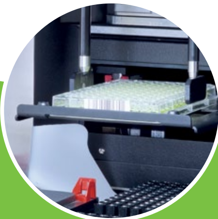
CO-RE Grippers transport microplate to microplate washer
